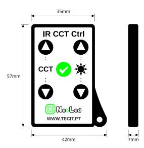
Infrared remote control to adjust the color temperature and luminous intensity of the 24v LED Bars.
